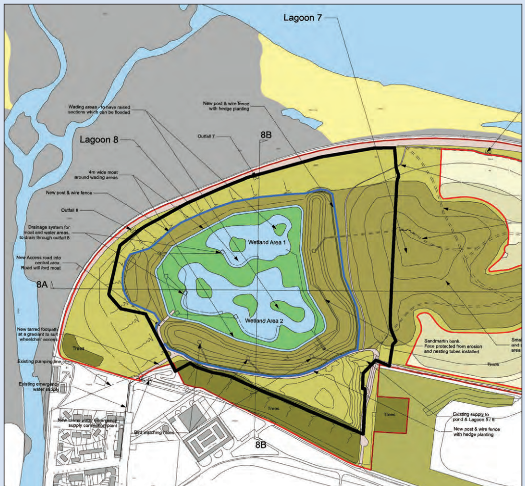
Figure 1. Extract from Scottish Power's plans for the westernmost lagoon at Musselburgh as approved on 3 October 2018. In addition, the solid black line denotes the limit of the Special Protection Area ( sitenlink.nature.scot/site/8499 ) and the new fence line is highlighted by a blue line. As downloaded from East Lothian Council's website: pa.eastlothian.gov.uk Reference 18/00388/PM. Note: a fifth hide (not shown) will be situated to the west of the new wetland.
